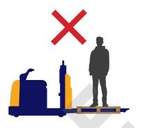
**Never** carry unpalletised goods (or any other unpalletised items) directly on the forks or footplate. A pallet, cage or attachment must be used.
