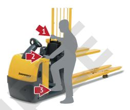
After mounting, adjust the tiller arm or steering adjuster to the correct operating position so hand controls will be easy to reach.
