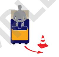
When manoeuvring laden, your field of view may be reduced, as may the space within which the truck has to operate. Bear this in mind.
